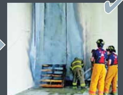
Result: Pass 25 ft. High Corner Test
